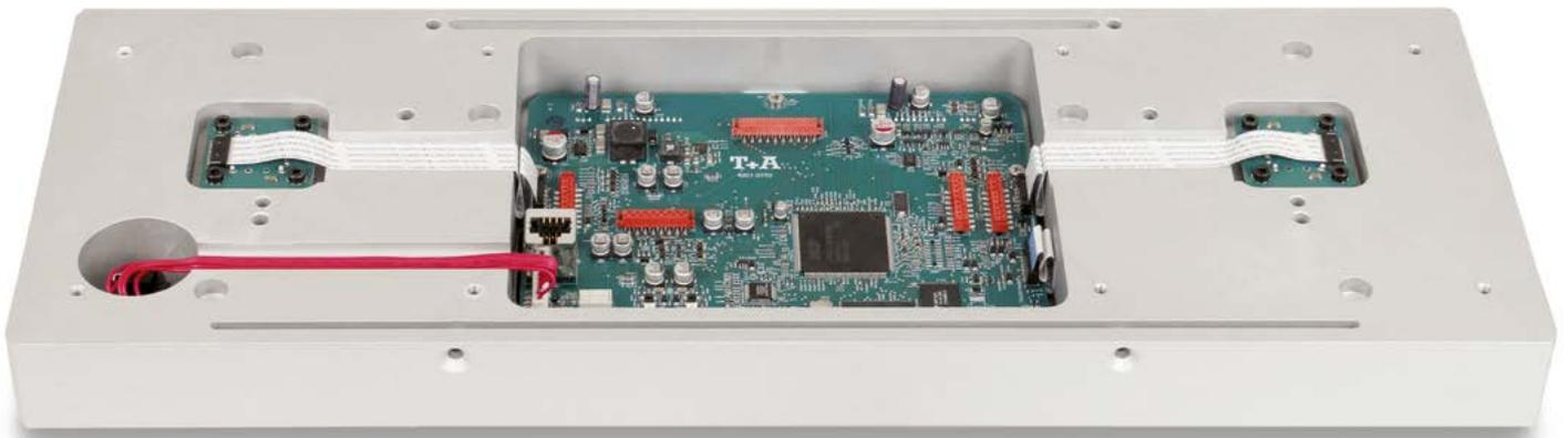
Non-magnetic materials are employed for all components and case parts, because this completely eliminates any chance of magnetically induced signal distortion. Such distortion can result in discoloration and degradation in the sound. All the essential chambers, supports and openings are produced using the latest milling machines, utilising a single process in order to
