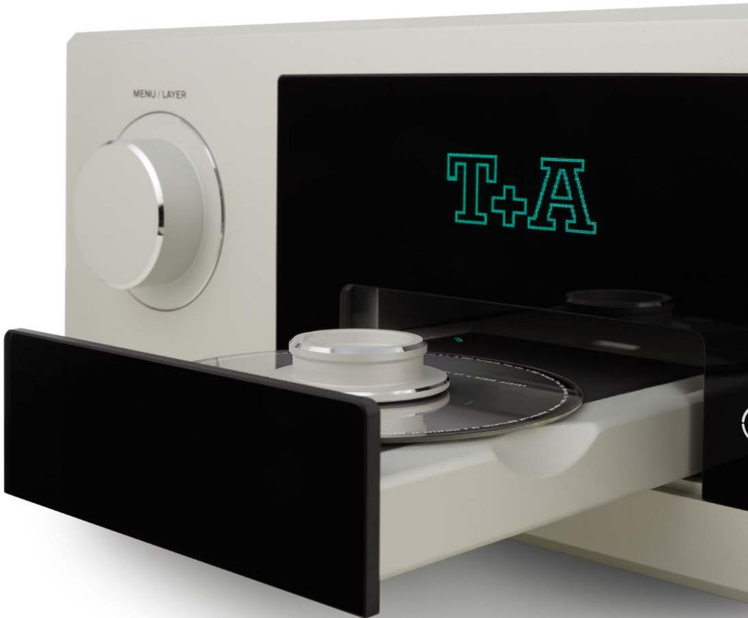
The High End loader unit of the PDT 3100 HV is machined from a single block of aluminium, 25 mm thick. All the drive mechanism components are installed in this heavy block, whose substantial mass isolates it from the remainder of the case. The whole block runs on two polished linear guides made from stainless steel, and is gently opened and closed by a spindle drive system.
