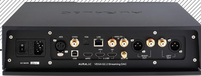
ABOVE: Digital inputs on AES, coaxial and optical (192kHz/24-bit and DSD64 over DoP) are joined by wired LAN, USB-B and Auralic Lightning Link ports (384kHz/32-bit and DSD512) plus an external clock input. Line inputs (on RCAs) sit alongside fixed/variable preamp outputs on XLRs (balanced) and RCAs
